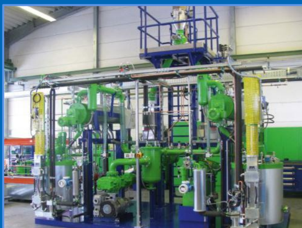
Filling Epoxy Resin in Vacuum Resin Casting Equipment
